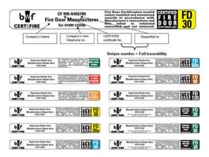
Building Regulations state that a front door to a flat must be **FD30S**. This means that the door needs to be 30 minute fire and smoke resistant, FD = Fire Door and 30 = relates to the minutes of fire resistance, S denotes that the door is also smoke sealed.
