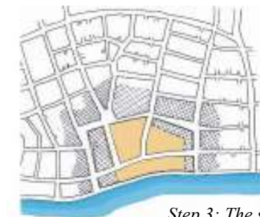
Step 3: The street pattern forms the basis for perimeter blocks within the development
