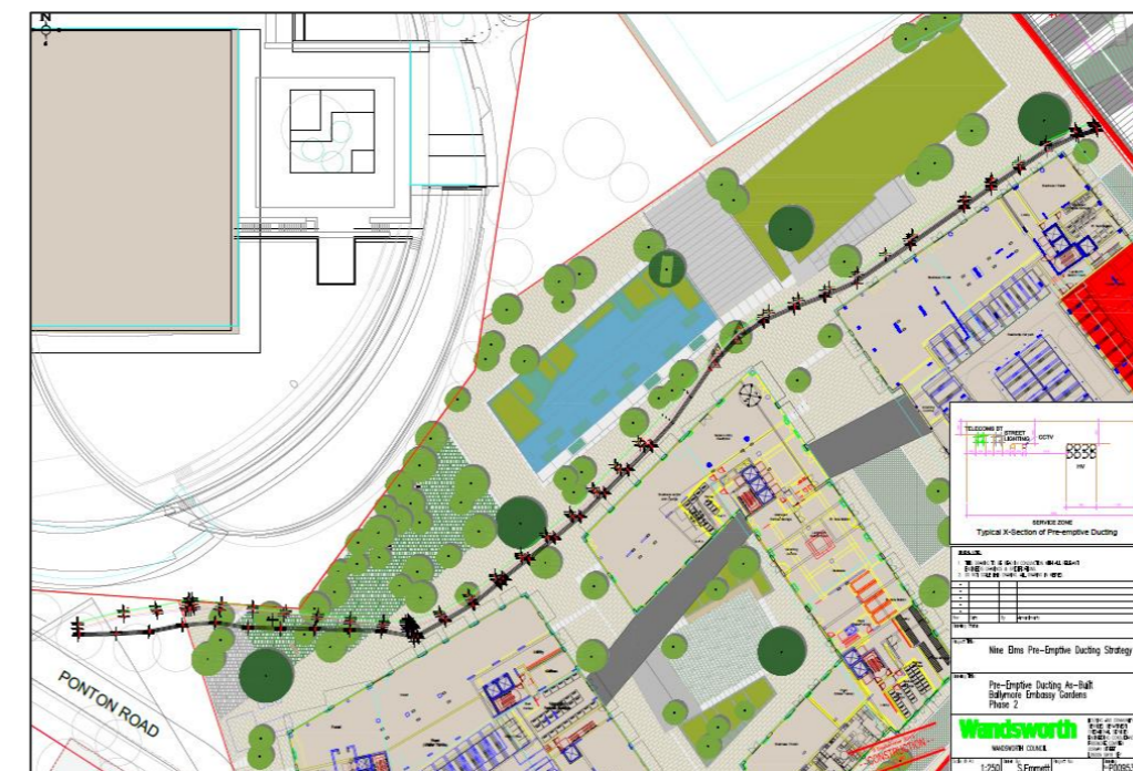
Figure 6.3: Pre-Emptive Ducting As Built – Ballymore Embassy Gardens Phase 2
