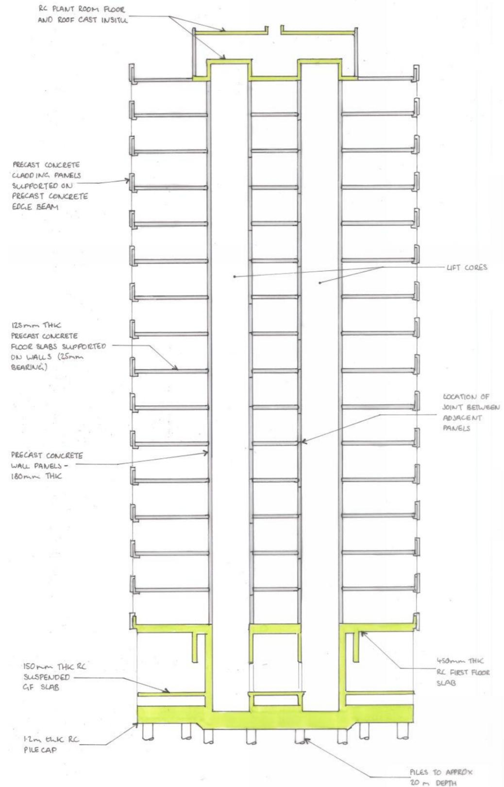
Figure 2.1: Section through tower showing existing structure
